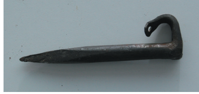
Early wrought-iron Mauershaken from c1880 and c1890 associated with the Zsigmondy brothers and Schmitt. Early pegs were simply metal-ware manufactured for other purposes that proved useful to alpinists. ( Messner Museum )
