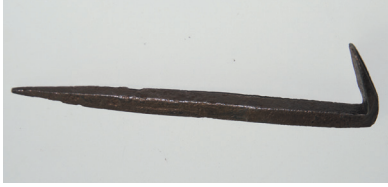
Early wrought-iron Mauershaken from c1880 and c1890 associated with the Zsigmondy brothers and Schmitt. Early pegs were simply metal-ware manufactured for other purposes that proved useful to alpinists. ( Messner Museum )
