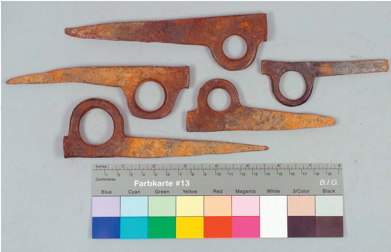
Fiechtlhaken, named for the innovative equipment designer Hans Fiechtl (1884-1925). These are likely not pre-First World War but typical of the pitons Fiechtl was manufacturing and sharing.
