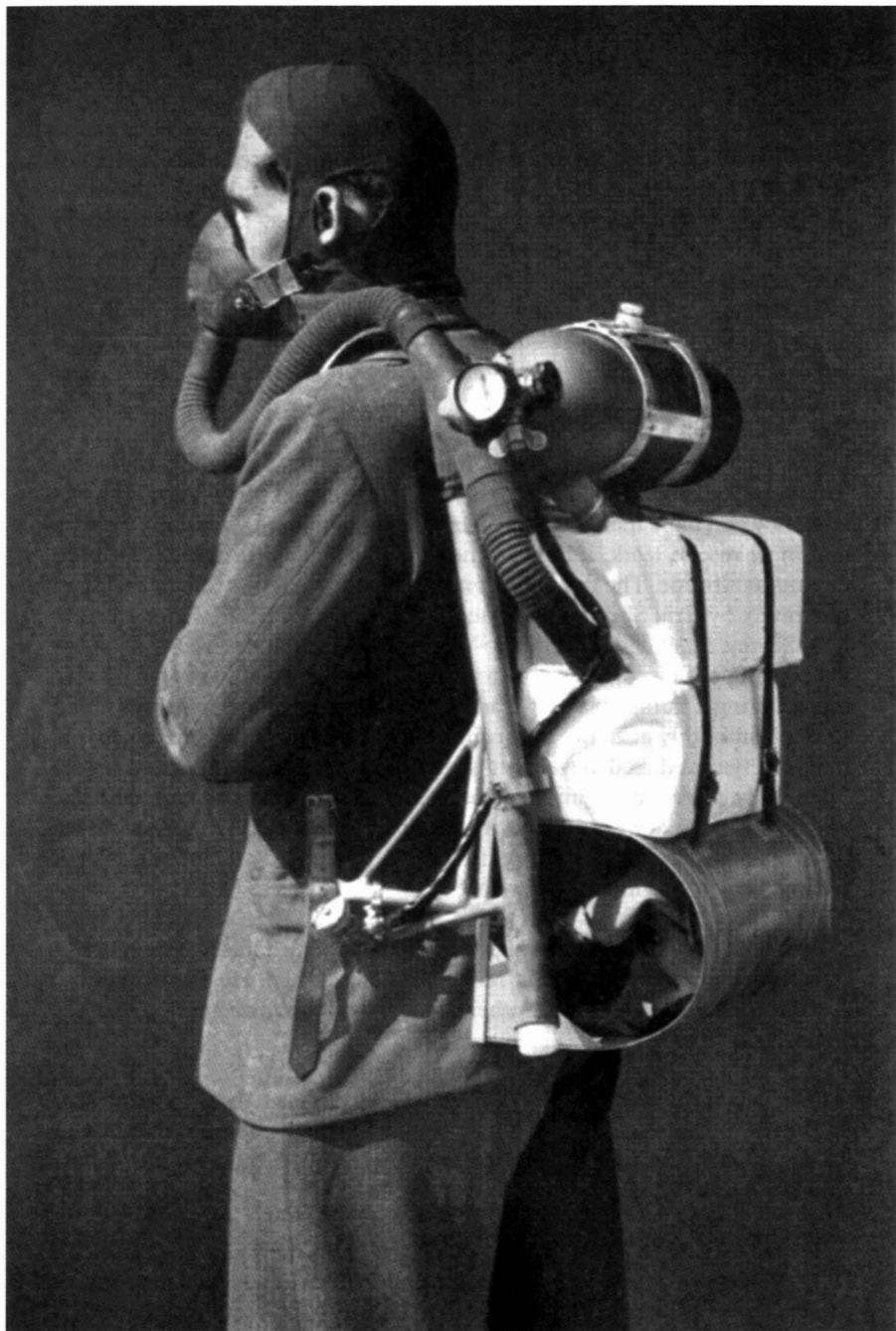
146. The closed-circuit oxygen set developed for use in 1953. (Alpine Club Photo Library)
